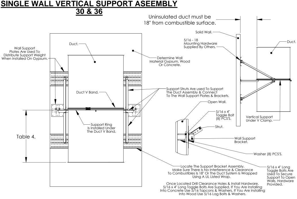
The Duct V Band Should Be Installed Above The Support Ring To Allow Vertical Movement.
